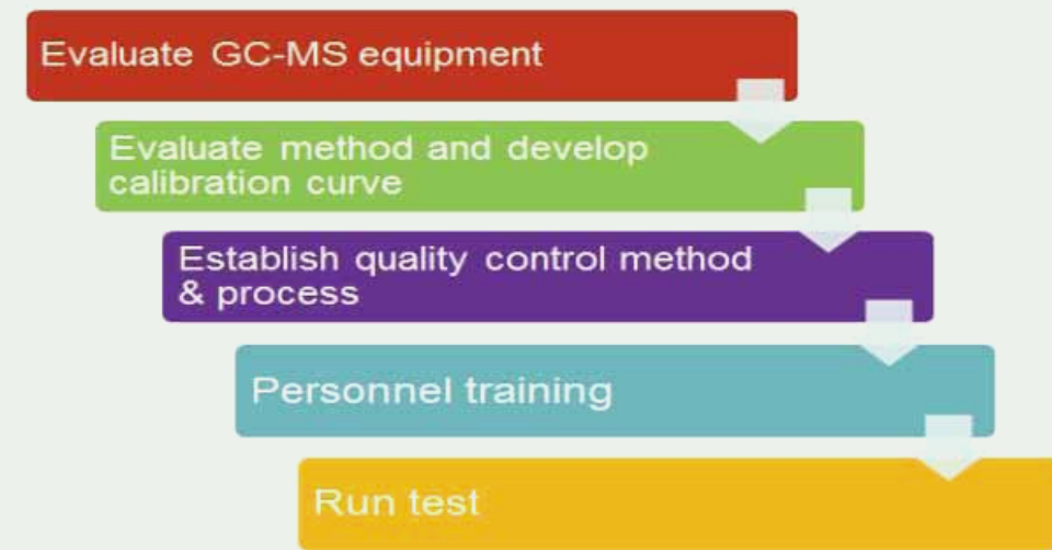
GC/MS phthalates inspection ability and method development processes
